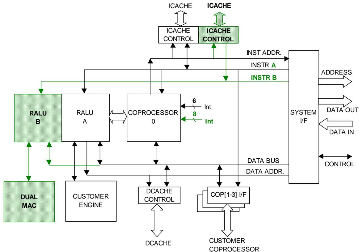
▶ **A configurable processor subsystem for SoC design**
